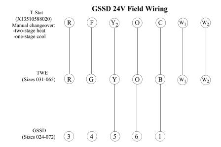
Figure 5: Field wire connections.
